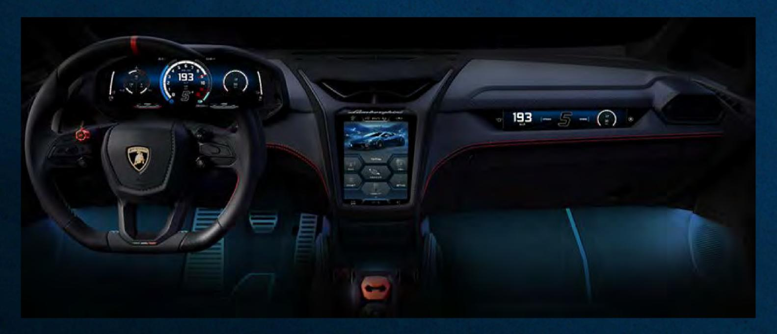
created specifically for Temerario, including 3D elements, animations, and widgets. The new HMI is also highly customizable, offering three view options: "Dynamic View" for vehicle dynamics information, "Navi View" for a full-screen map, and "Essential View" for basic driving information. The Infotainment can be customized at will to create a fully immersive experience based on the user's preference.
